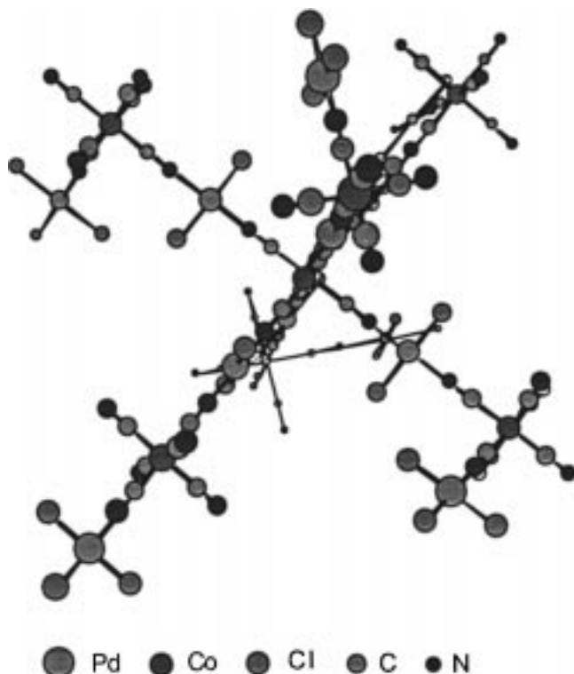
Figure 1. Proposed star polymer structure of cyanogel polymer network.
